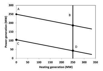
$Power_{chp,i} \leq PowerCapacity_{chp} - StorageInput_{chp,i} \cdot CHPPowerLossFactor_{chp}$   $Power_{chp,i} \geq PowerMustRun_{chp,i} - StorageInput_{chp,i} * CHPPowerLossFactor_{chp}$
