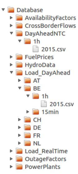
The above figure shows a partially unfolded view of the database structure. In that example, data is provided for the day-ahead net transfer capacities for all lines in the EU, for the year 2015 and with a 1h time resolution. Time series are also provided for the day-ahead load forecast for Belgium in 2015 with 1h time resolution.
