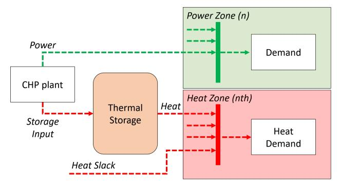
The following heat balance constraints are used for any CHP and P2H plant types.
