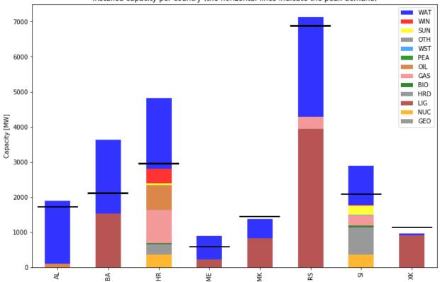
Installed capacity per country (the horizontal lines indicate the peak demand)
